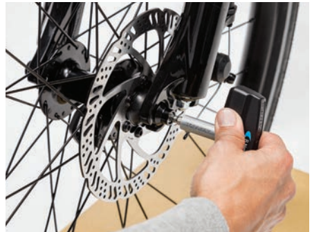
Figure Loosening axle bolt
