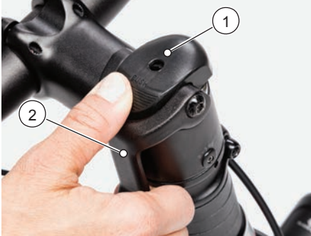
Figure Opening stem Lever
