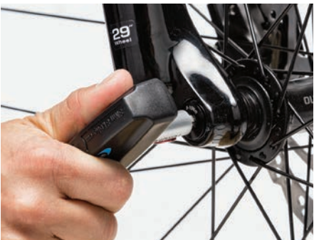
Figure Loosening the thru-axle.
