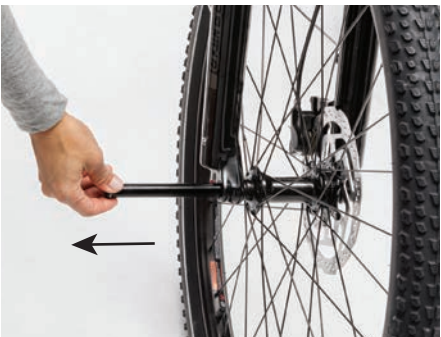
Figure Sliding out the thru-axle
