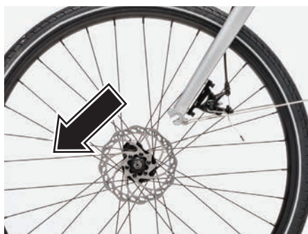
Figure Removing wheel front dropout.
