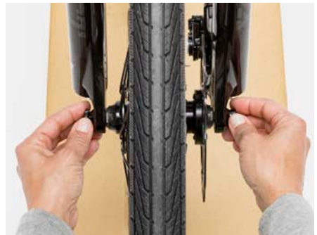
Figure Un-threading axle nut
