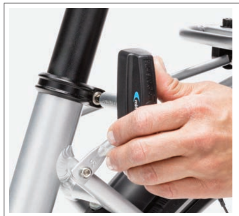
Figure Loosening the seat binder bolt.
