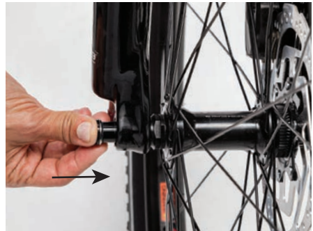
Figure Aligned fork dropouts and wheel hub.
