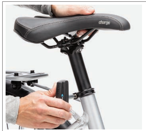
Figure Setting the saddle height
