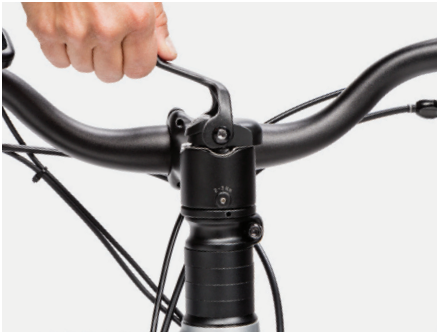
Figure Stem lever open
