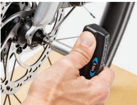
Figure Torque (tightening) with the Charge torque tool.
