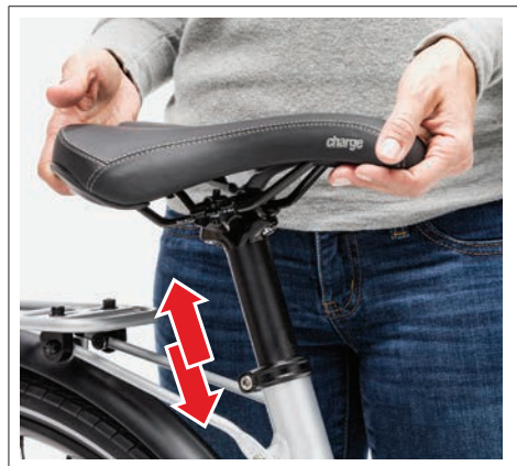
Figure Setting the saddle height
