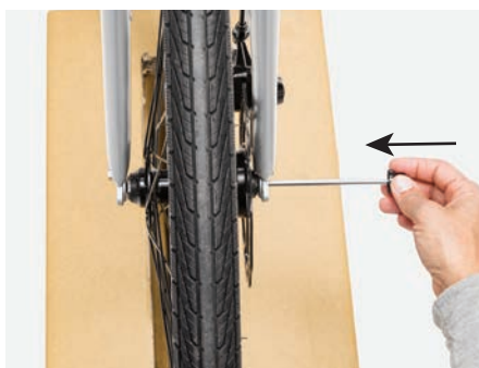
Figure Inserting axle into wheel hub.
