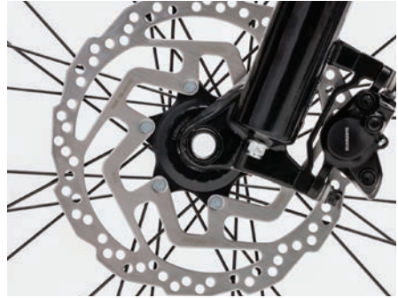
Figure Aligned fork dropouts and wheel hub hole.
