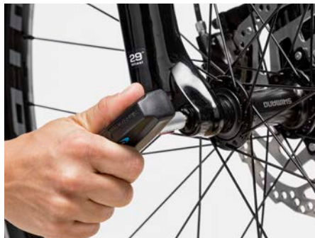
Figure Torque (tightening) with the Charge torque tool.
