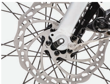
Figure Lowering fork dropouts onto wheel.
